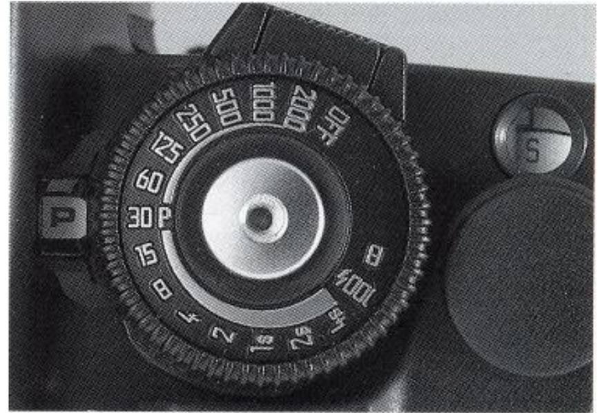
When using non-system flash units, the shutter speed must be set to "100~~⚡~~". In the "B" setting, the shutter remains open for as long as the exposure release button is pressed down. The symbol "bulb" is displayed in the viewfinder.
