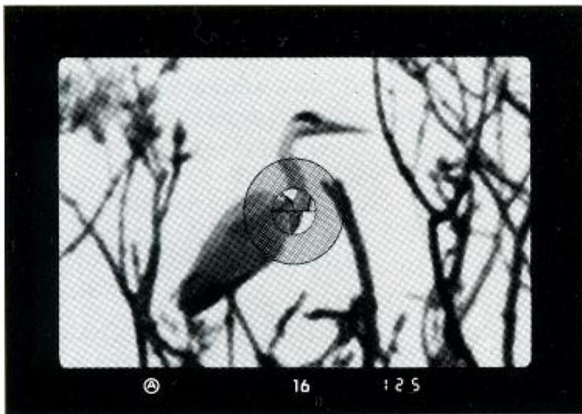
The remainder of the screen looks like a ground-glass screen and is ideal for focusing telephoto lenses and for close-range photography.
