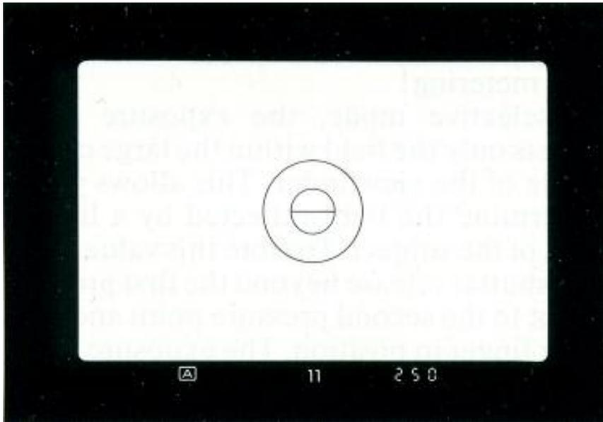
In extreme brightness, the shutter speed range may not be sufficient for correct exposure, indicated by "2000" flashing. Simply set a smaller aperture. Conversely, if, in poor light, the "16", symbol flashes, a larger aperture should be set to prevent under-exposure.
